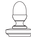
AF/70/PC acorn finial and post cap for PO/70 125 x 125 x 155mm (5in x 5in x 6in)
